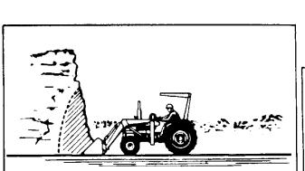
Exercise caution when undercutting high banks. Dirt slides can be dangerous. Load from as low as possible for maximum efficiency. Loader lift and breakaway capacity diminish as loading height is increased.
